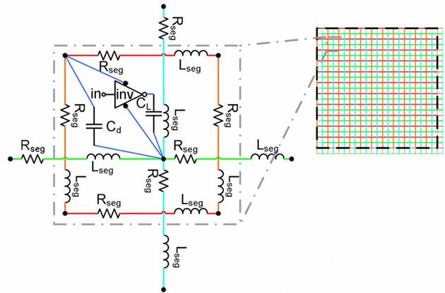
Fig. 4 In order to facilitate the P/G network analysis, each wire segment is modeled as a chain of L-type RLC equivalent circuits. An inverter with a capacitance load is used to imitate the core logic. A decap is connected to the intersection points on the vdd/vss grids [21]
