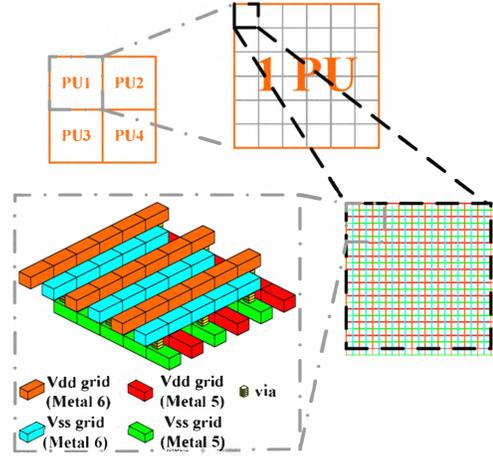
Fig. 3 P/G network architecture of each tier [21]
