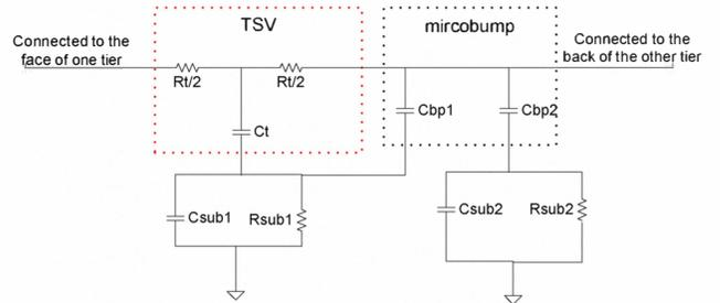
Fig. 7 Vertical interconnection model using Face-to-Back bonding [22]
