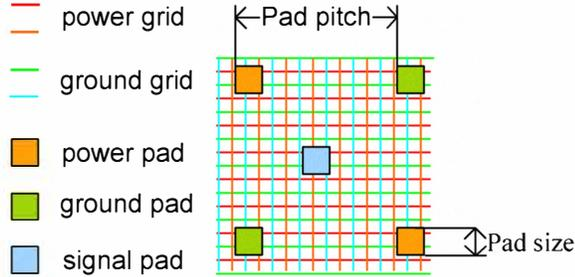
Fig. 5 On-chip power/ground grids and I/O pads on the bottommost die
