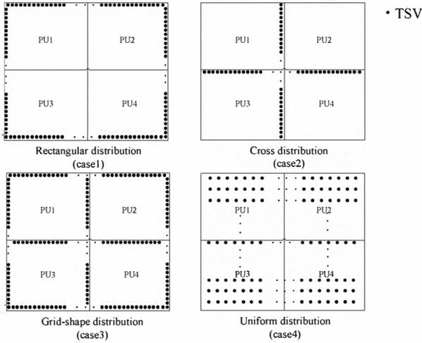
Fig. 8 Different TSV distributions for one layer
