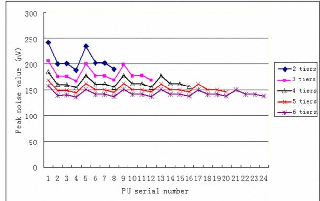
Fig. 9 Simulation results for different number of tiers ( the serial number of  $PU_i$  in tier  $j$  is  $i+(j-1) \times 4$ )
