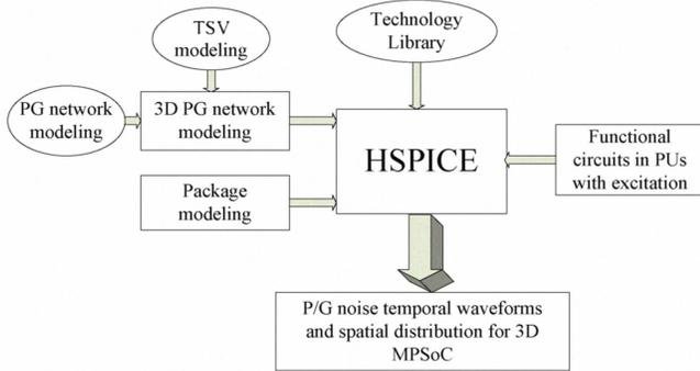
Fig. 1 Power Gating induced P/G noise analysis platform for 3D MPSoC
