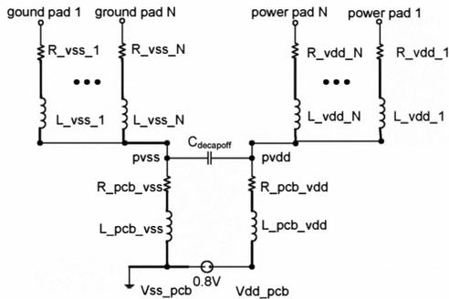
Fig. 6 Package model with package L and off-chip decoupling capacitance
