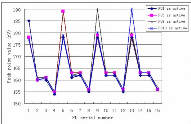
Fig. 10 Simulation results when different PUs are active (the serial number of  $PU_i$  in tier  $j$  is  $i+(j-1) \times 4$ )
